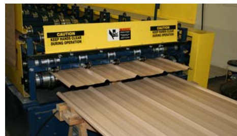
Step 4 Roll Forming Process Finished Panel
